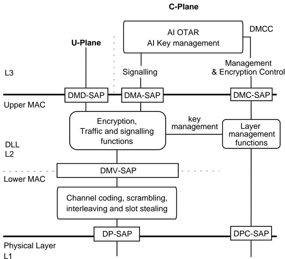
Figure 14: Relationship of security functions to layer functions
