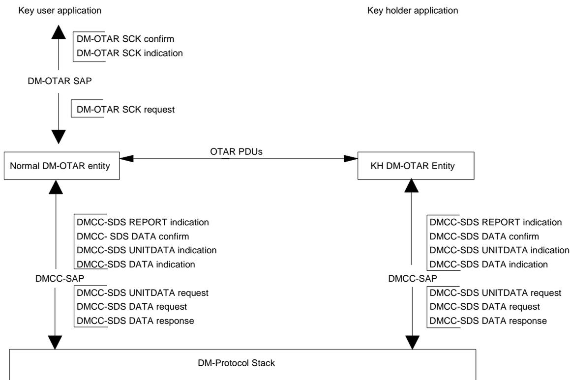
Figure 19: Model for MS to KH protocol
