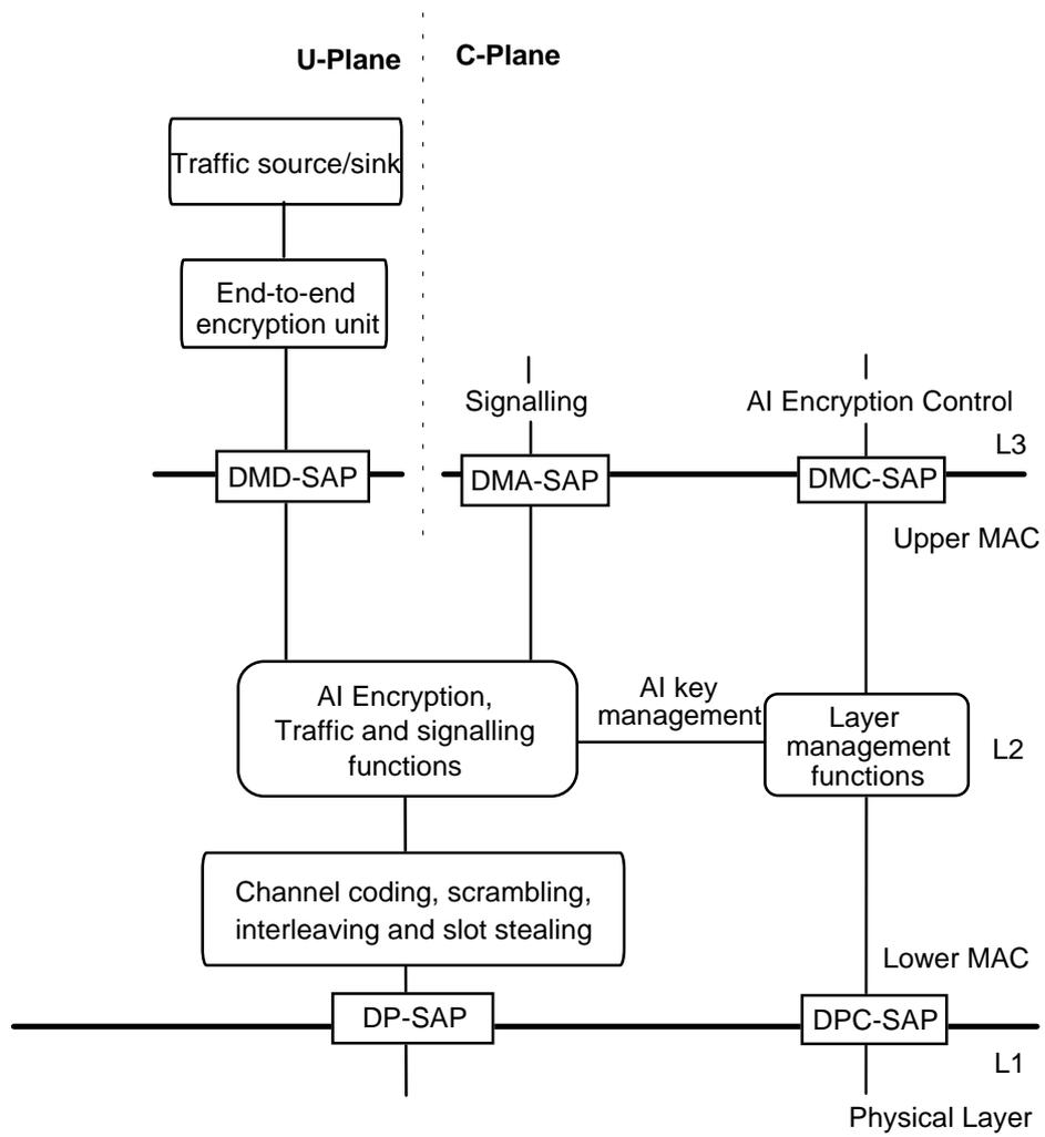
Figure 39: Position of end-to-end encryption unit in MS
