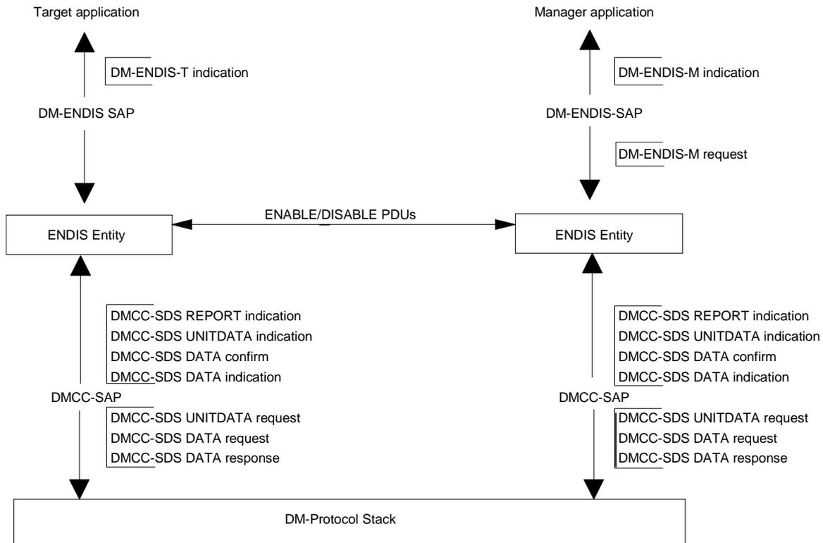
**Figure 30: Model for manger to target protocol**
