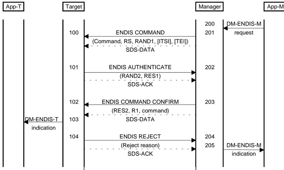
Figure 35: Treating authentication failure during ENDIS exchange
