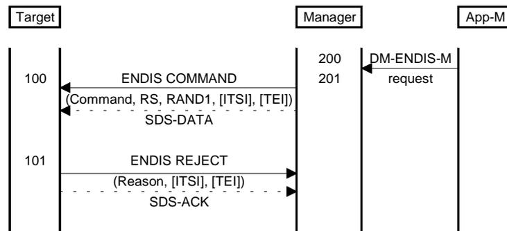
**Figure 34: Rejecting a command**
