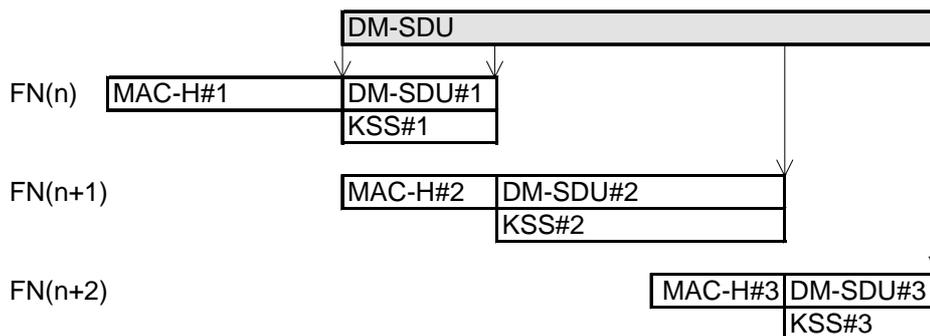
NOTE 1: The example DM-SDU is fragmented over 3 slots by breaking it into DM-SDU#1, DM-SDU#2 and DM-SDU#3
