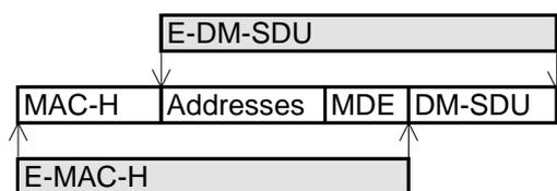
**Figure 10: Concatenated structure of TETRA DMO elements**
