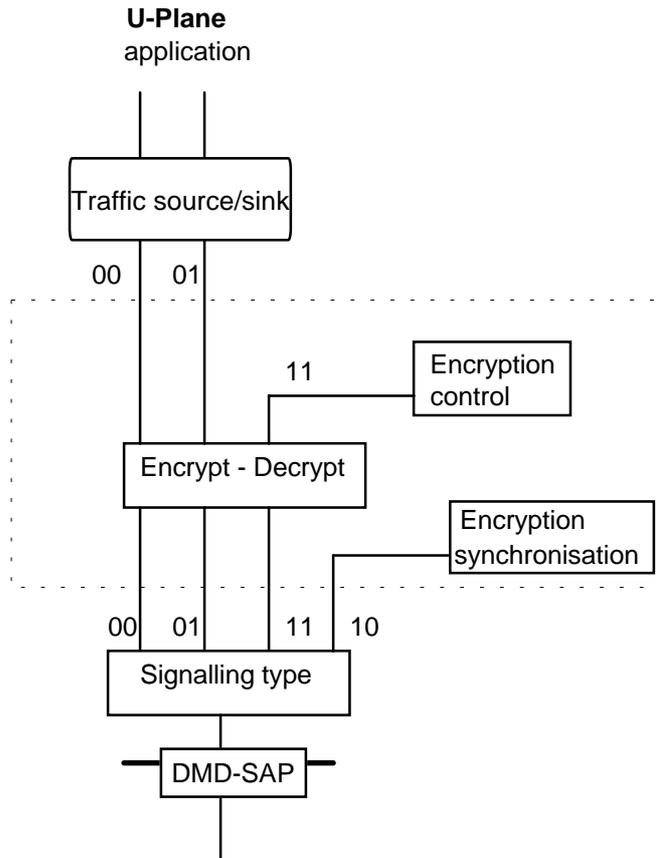
Figure 40: Functional model of the encryption unit
