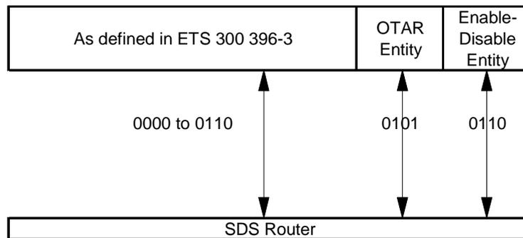
Figure 29: Routing of SDS messages to terminating entities
