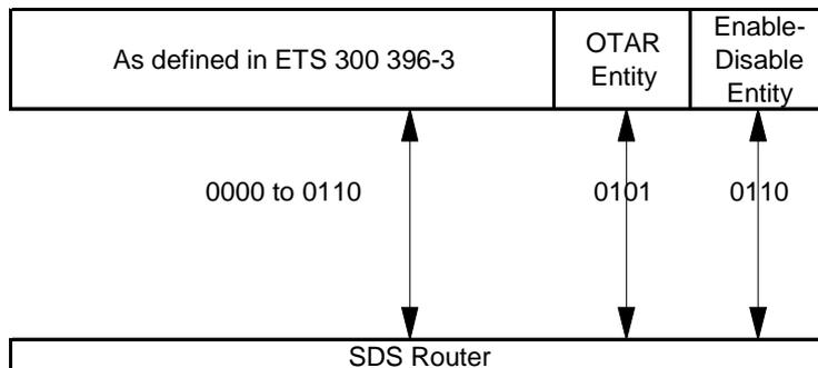
Figure 18: Routing of SDS messages to terminating entities
